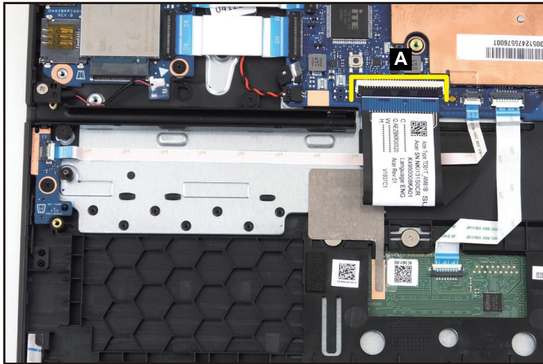
Figure 1-9. Power Board Removal
